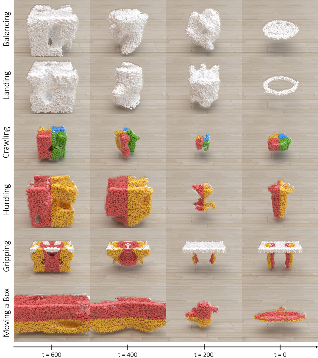
Figure 5: Demonstrations of generations changing from noises to robots with physical utility throughout the diffusion sampling process. We present snapshots at diffusion times t = 600, 400, 200, 0 for all presented tasks.
