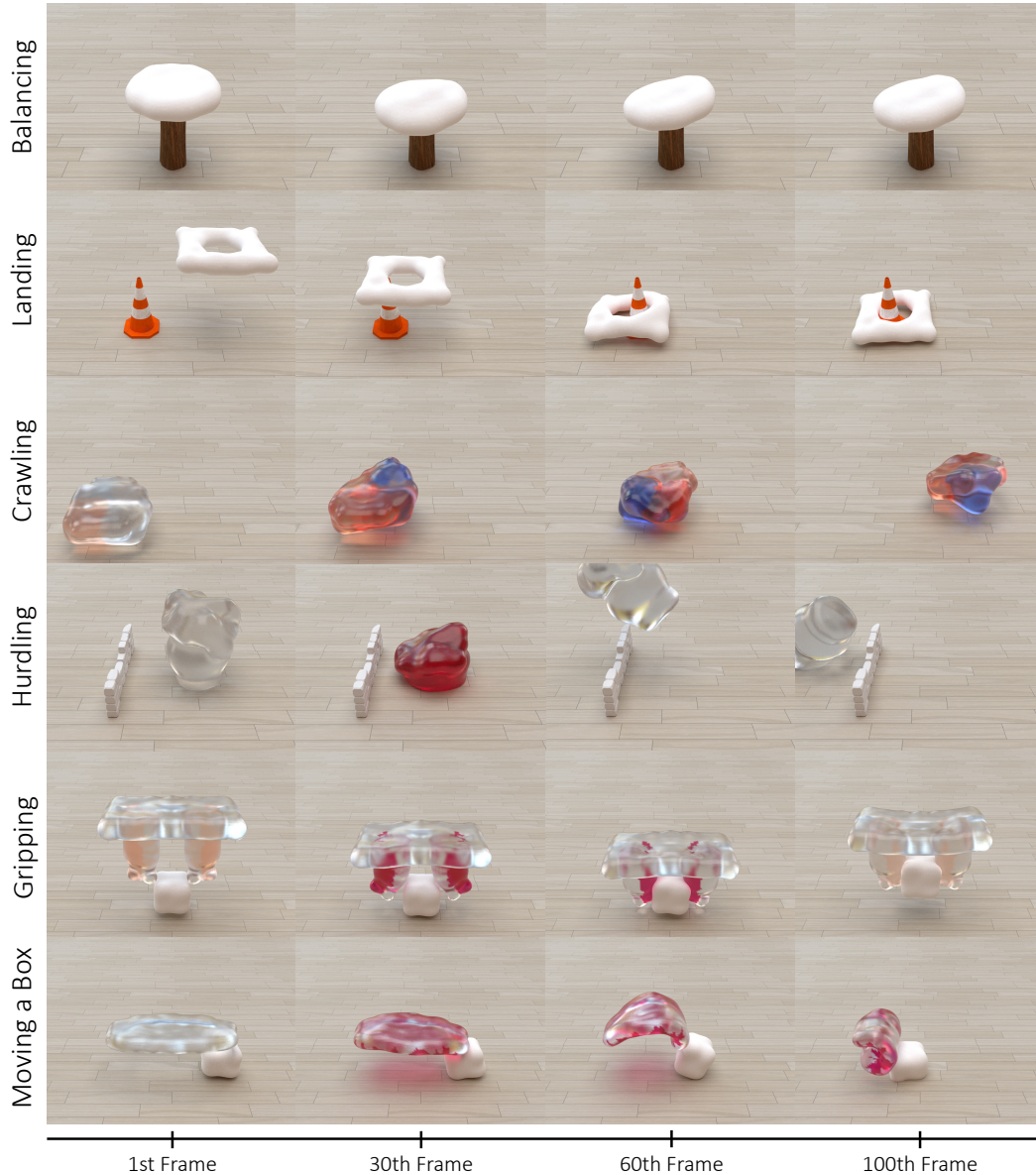
Figure 3: Examples of robots bred by DiffuseBot to achieve the all presented tasks.
